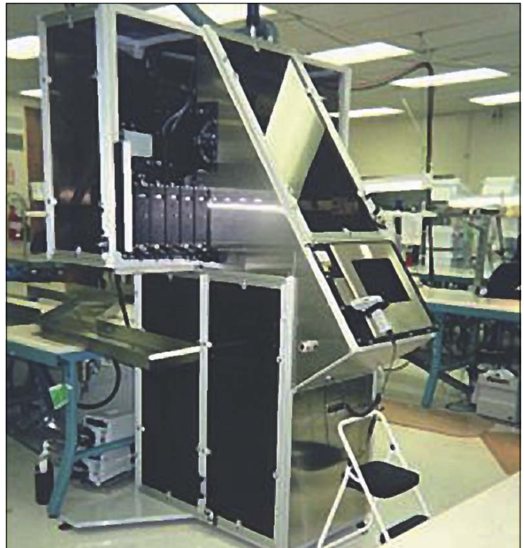
Figure 4-4 A pulsed UV system for curing lubricious coatings on medical guide wires is integrated into an automated production environment. (Photo courtesy Guidant Corporation)
