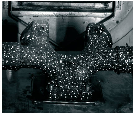
DIC measurements of a hot (800°C) exhaust manifold - with filter (left) and without filter (right) Acknowledgement: images taken during a project with KTH Royal Institute of Technology (Sweden) and Scania.
