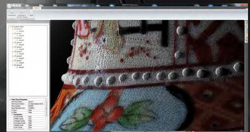
3D scanning result: colour cloud of points with 700 pts/mm 2
