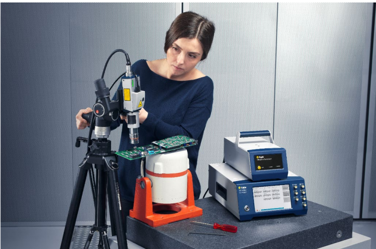
Figure 2: Non-contact measurement of vibrations even on the finest structures, e.g. for reliability testing of electronic components with the VibroFlex Compact with microscope optics, coaxial illumination unit and HD+ camera for visual control and documentation.
