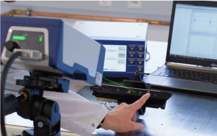
Figure 1: Laser-based vibration measurement with VibroFlex Xtra is perfect for dark, moving or rotating surfaces – here being used to test the haptic feedback of an automotive control panel.
