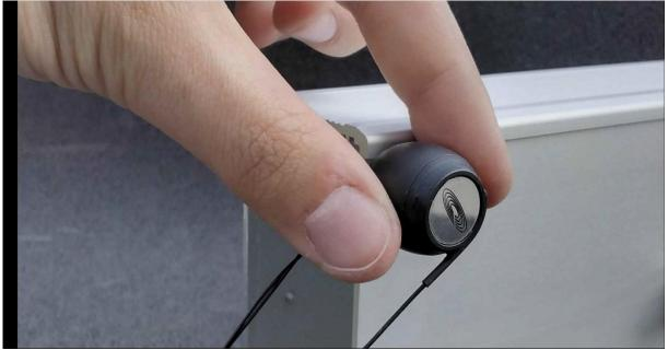
The Qlws LightWeightShaker is self-supporting and can be attached in any direction to the device under test for consistent vibration excitation in experimental modal tests.
