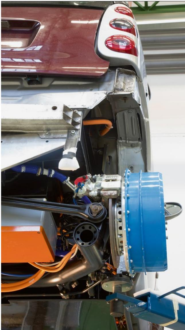
**FIGURE 1** Wheel hub motor implemented in the research vehicle Editha 3
