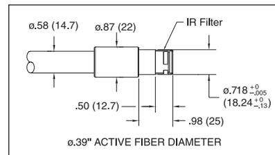
All standard PANELite® backlight configurations have the same input dimensions.
