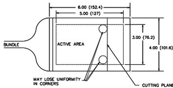
The A23000 PANELite® backlight can be trimmed in either direction with a good pair of scissors.
