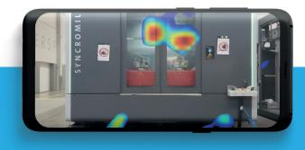
State-of-the-art machine tools exhibit a wide variety of complex sound events during the machining process. Engineers working in product development trust in the visualization of sound radiation in order to take quick and effective measures to comply with noise limits.
