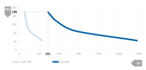
Calculation of the lowest frequency (Hz) at 180° opening angle (DEG)
