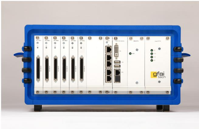
The mcdRec is the heart of the basic Acoustic Camera Pro system, which also consists of a microphone array, and a notebook or other workstation with the NoiseImage analysis software.
