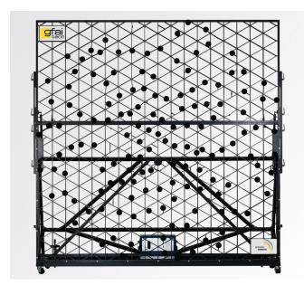
The mobile array Evo was developed specifically for use in aeroacoustic applications, namely wind tunnel testing. The array's foldable construction simplifies handling, transport and storage. The back frame is conveniently used as a storage area for the data recorder to ensure high mobility and compactness of the entire measurement system. Ground anchor points also help stabilize the system during measurement.
