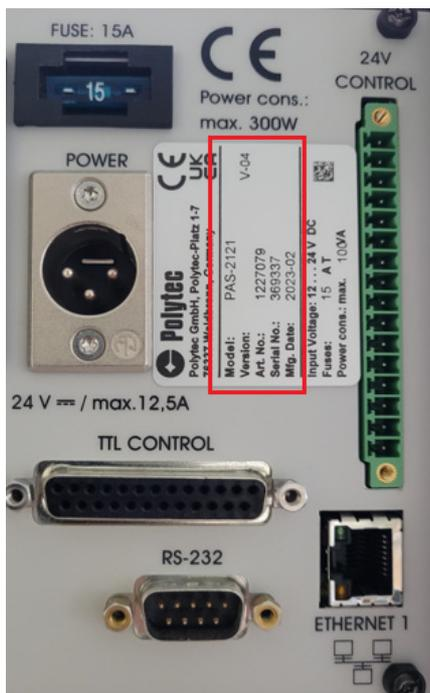
Figure 1: Name plate with serial number on the back of the spectrometer
