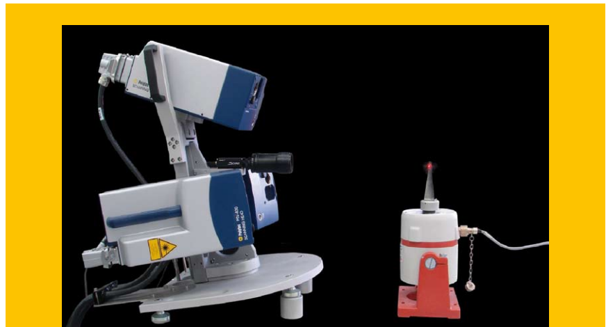
Fig. 2: 3-D Scanning Vibrometer testing a turbine blade.
