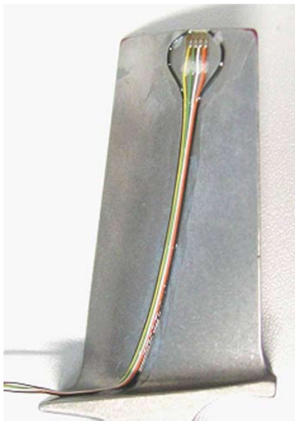
Fig. 1: Instrumented turbine blade with strain gauges.
