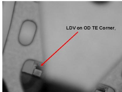
Figure 2: LDV on trailing edge orner (outside diameter).
