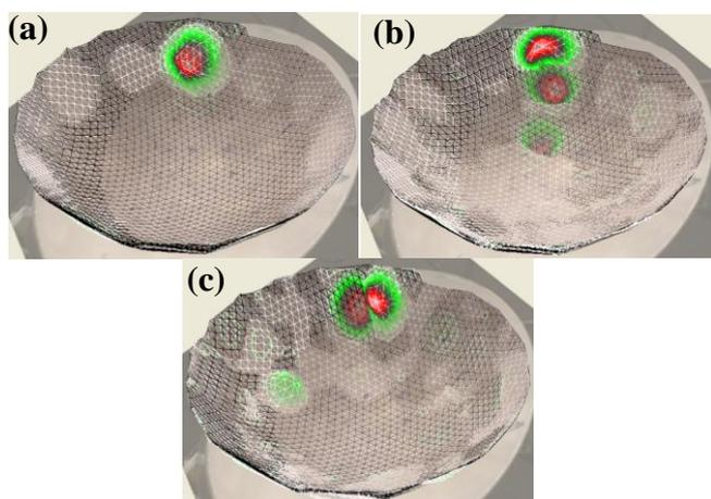
**Figure 4:** First three flexural modes of C4<sup>#</sup> note region: (a) 276Hz, (b) 550Hz and (c) 640Hz
