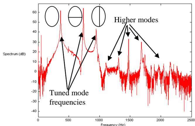
**Figure 6:** Typical frequency response spectrum for outer note on the soprano pan. First three modes are usually tuned into a nearly harmonic relationship. Higher modes are not harmonic but contribute to the overall timbre of the steelpan. Obtained using 1D scanning laser Doppler vibrometer and excitation using an impact hammer.
