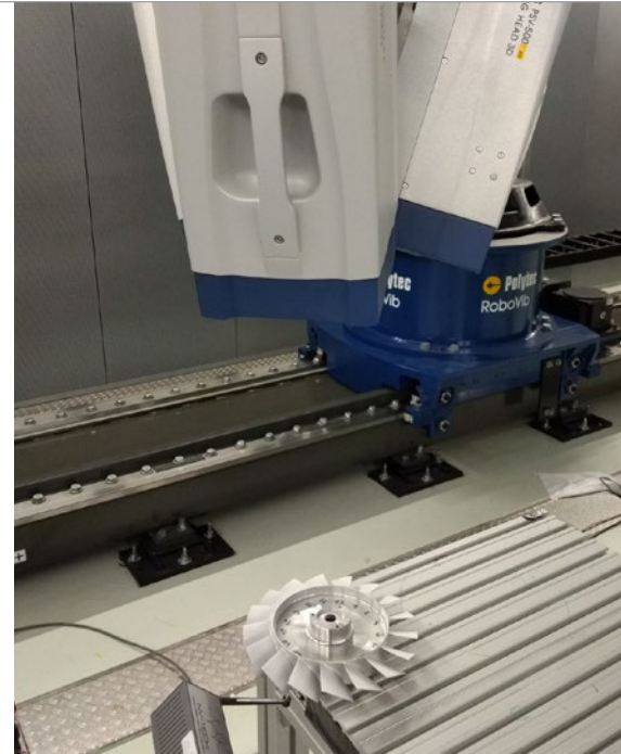
Figure 1: Measurement setup of a 3D Scanning Laser Doppler Vibrometer on a blisk of 240 mm diameter
