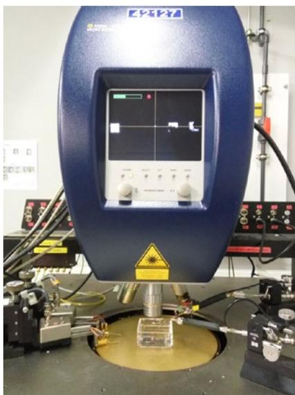
Figure 2: Schematic of the experimental set-ups: (a) Optical set-up for the dynamic characterization using a Polytec vibrometer system; (b) Acoustic set-up for the sound pressure measurements using a hydrophone.
