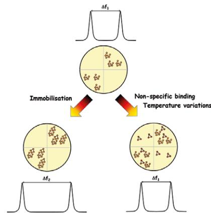
Figure 2: Upon functionalization of the sensor, degeneracy is broken and the modal frequencies show a split of  $\Delta f_1$ . Addition of mass to the antinodal position of the functionalized mode increase this split to  $\Delta f_2$ . For non specific variations, the split remains unaltered.
