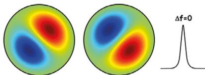
Figure 1: The mode shapes for the (1,0) vibration of a circular diaphragm. For a symmetric device, the modes form a degenerate pair.
