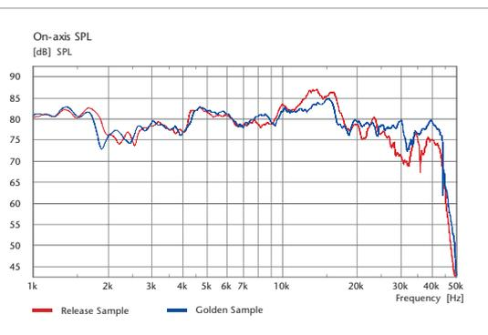
Fig. 1: On-axis Sound Pressure Level (SPL) spectra from tested BMR's.
