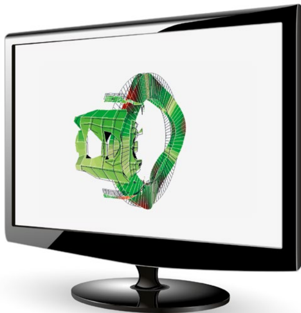
Analysis of both in-plane and out-of-plane motions for understanding complex dynamics, here on an automotive brake.
