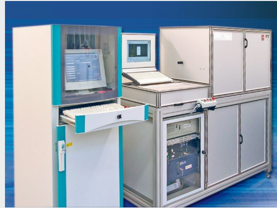
3 Complete test station for 100% quality control of nebulizer membranes
