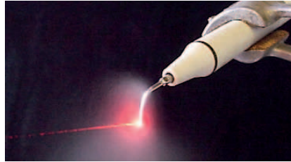
The laser of the scanning vibrometer measures the surface of a dental ultrasonic scaler.
