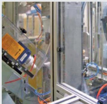
**Figure 3:** Protective housing with air wipe for the IVS vibrometer
