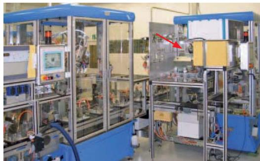
Figure 1: Automatic test station for motor pump assemblies (MPA). Mark: IVS vibrometer
