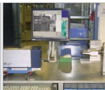
**Figure 3: Measurement layout to characterize the sonotrodes**
