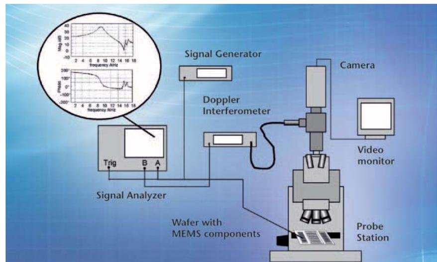
Figure 2: Probe station with Polytec Microscope Scanning Vibrometer
