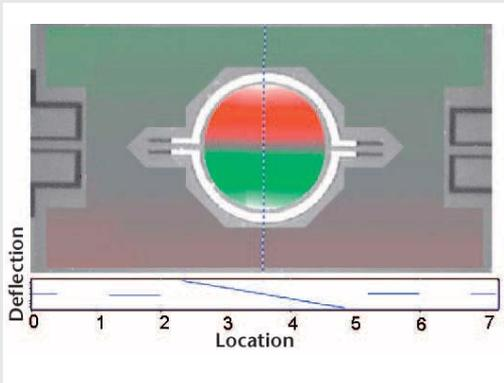
Figure 6.1: Measurement results with the Microscope Scanning Vibrometer: deflection shape
