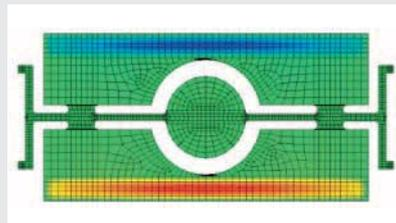
Figure 4: FEM analysis of damping by air flow, pressure distribution
