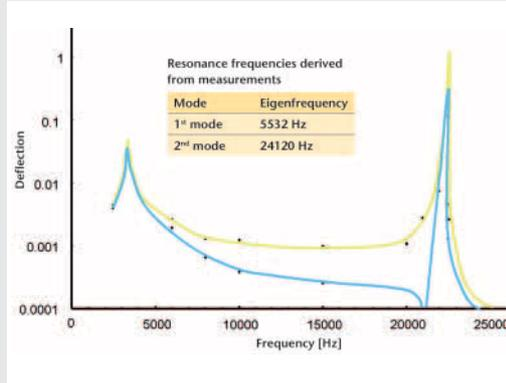
Figure 6.2: Measurement results with the Microscope Scanning Vibrometer: transfer function
