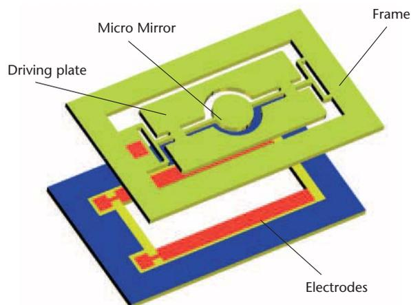
Figure 1: Construction of a micro scanner
