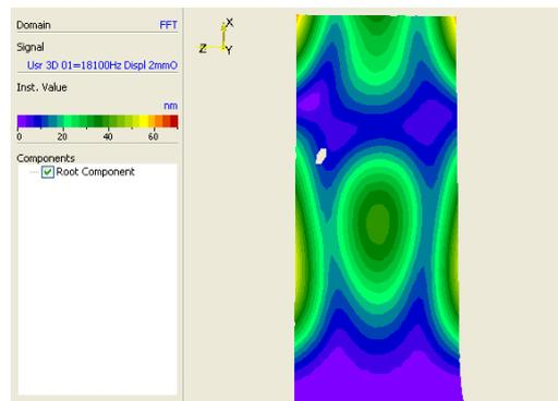
Fig. 5b) displacement at 18,100 Hz with VideoTriangulation.
