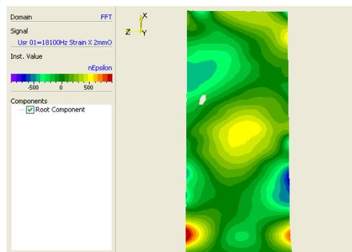
Fig. 5c) Strain along long axis at 18100 Hz without VideoTriangulation.
