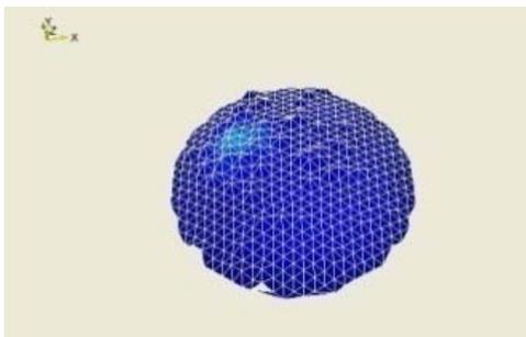
Fig. 3d) in-plane vibration at 102 kHz with VideoTriangulation.
