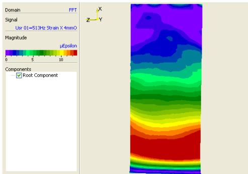
Fig. 4c) Strain along the long axis of the blade at 512 Hz without VideoTriangulation.
