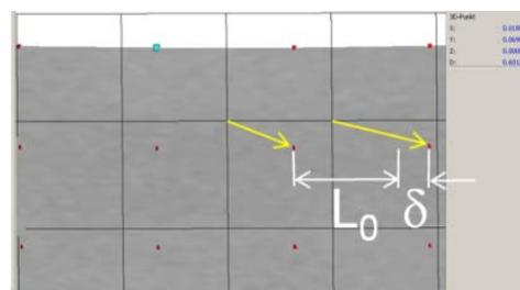
Fig. 2: Calculation of strain.
