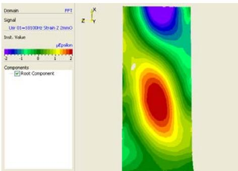
Fig. 5e) Strain along short axis at 18100 Hz without VideoTriangulation.
