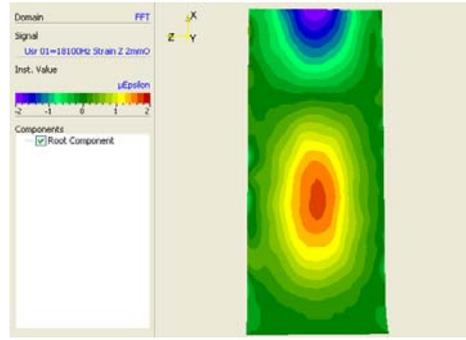
Fig. 5f) Strain along short axis at 18100 Hz with VideoTriangulation.
