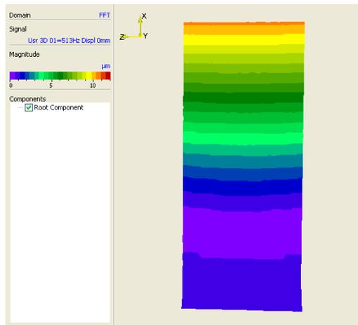
Fig. 4b) displacement at 512 Hz with VideoTriangulation.
