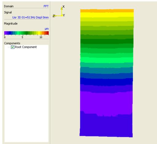
Fig. 4a) displacement at 512 Hz without VideoTriangulation.
