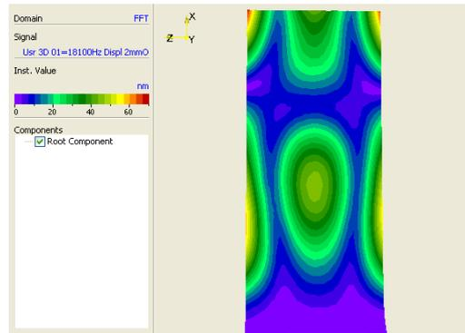
Fig. 5a) Displacement at 18100 Hz without VideoTriangulation.
