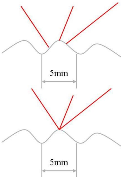
Fig. 1: beam intersection with standard 3-D coordinate measurement as compared to ideal case.
