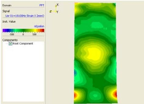
Fig. 5d) Strain along long axis at 18100 Hz with VideoTriangulation.
