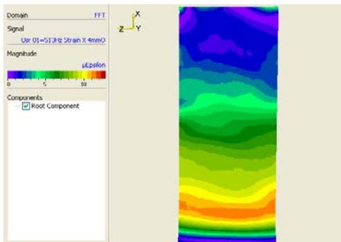
Fig. 4d) Strain along the long axis of the blade at 512 Hz with VideoTriangulation.
