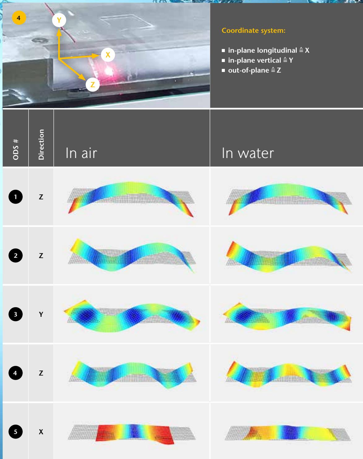
A closer look at the data shows the differences due to the presence of the surrounding water. The following Figures 5 and 6 show the average spectra of both measurements, left in air, right in water.
