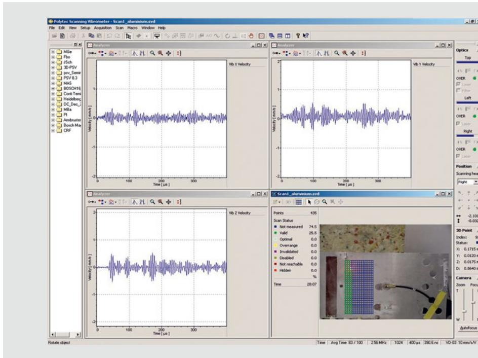
**2** In-plane and out-of-plane Lamb wave responses plotted using Polytec's PSV Software
