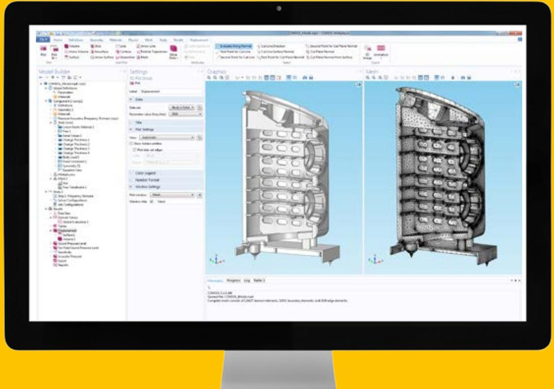
Geometry and mesh of the loudspeaker in the COMSOL GUI.
