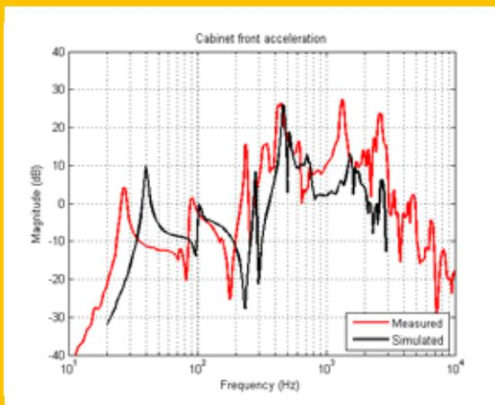
**Cabinet front acceleration as a function of frequency from simulation (black line) and measurement (red line).**
