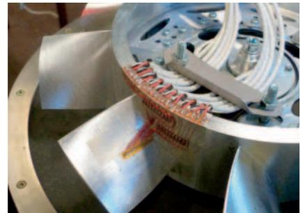
Fig. 1: Fan blade with strain gages in complete fan.
