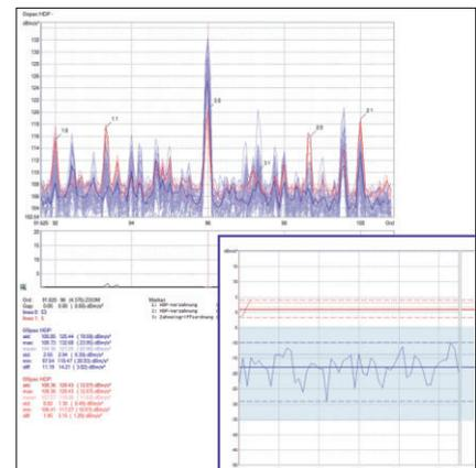
Fig. 2: Sideband energy measure based on order analysis for assessment of tothing vibrations.
