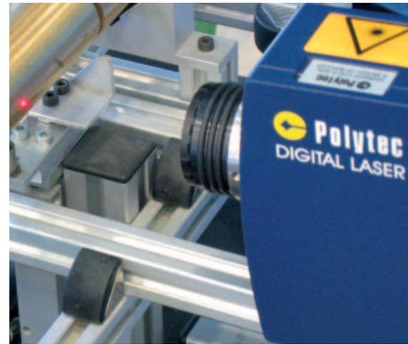
Fig. 2: IVS Industrial Vibrometer in a test stand at Polytec (not related to the application described here).
