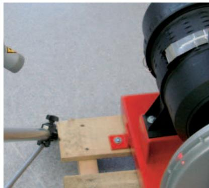
Fig. 1: Example of a measurement using a laser vibrometer to characterize an electric motor.
