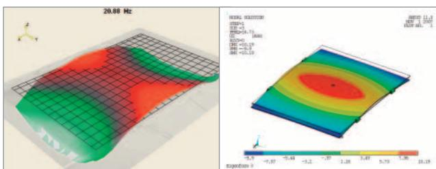
**Fig. 3: First ODS measured at 20.9 Hz (left) corresponding to the simulated mode at 18.7 Hz (right).**
