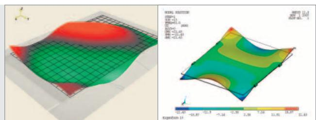
**Fig. 4: Third ODS measured at 63.8 Hz (left) corresponding to the simulated mode at 61.5 Hz (right).**
