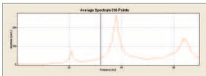
**Fig. 2: Frequency spectrum averaged over all 316 measurement points.**
