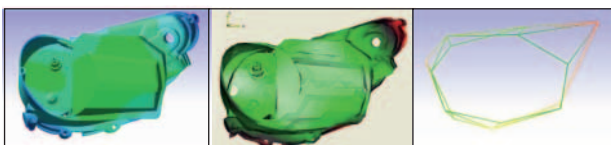
Fig. 4: Comparison of mode shapes from FE analysis (left) with RoboVib® (center) and conventional measurements (right).
