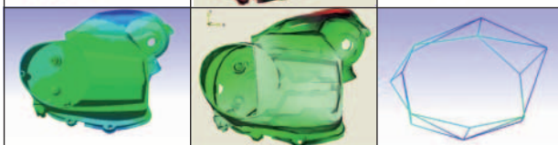
Fig. 4: Comparison of mode shapes from FE analysis (left) with RoboVib® (center) and conventional measurements (right).
