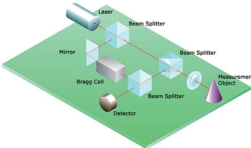
Figure 4: Optical configuration of a laser vibrometer [1]
