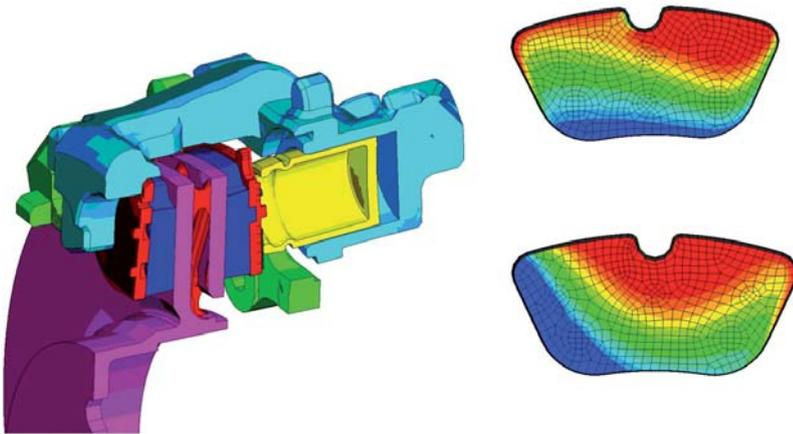
**Figure 2:** Presentation of the components (left) and calculation of deformation due to clamping and peripheral forces (right)
