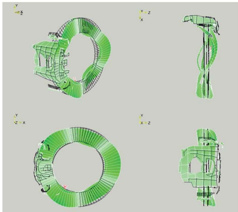
**Figure 8:** Measured operational deflection shapes
