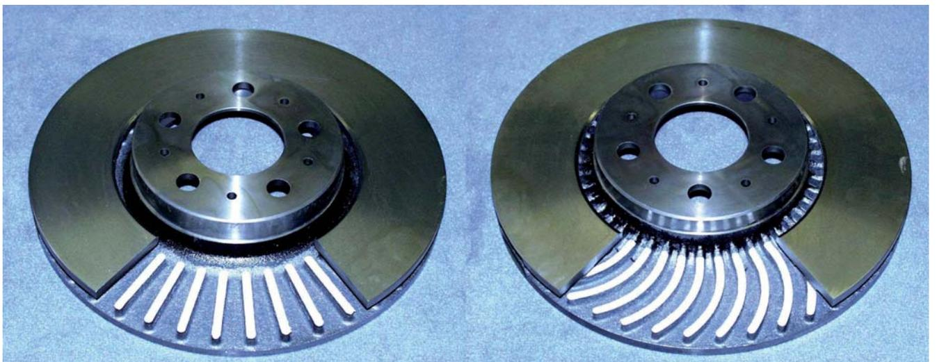
**Figure 11:** Structural imbalance due to modification of the disc stiffness (straight and bent cooling ducts)
