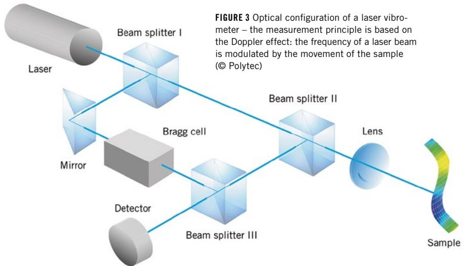
**FIGURE 3** Optical configuration of a laser vibrometer – the measurement principle is based on the Doppler effect: the frequency of a laser beam is modulated by the movement of the sample (© Polytec)
