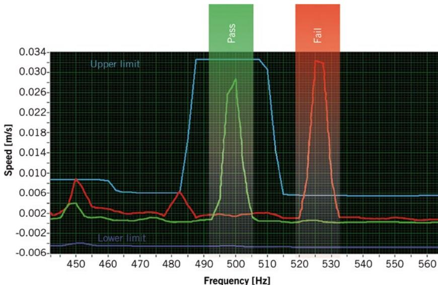
**FIGURE 2** Pass/fail decision by means of a deviating acoustic signature (© Polytec)
