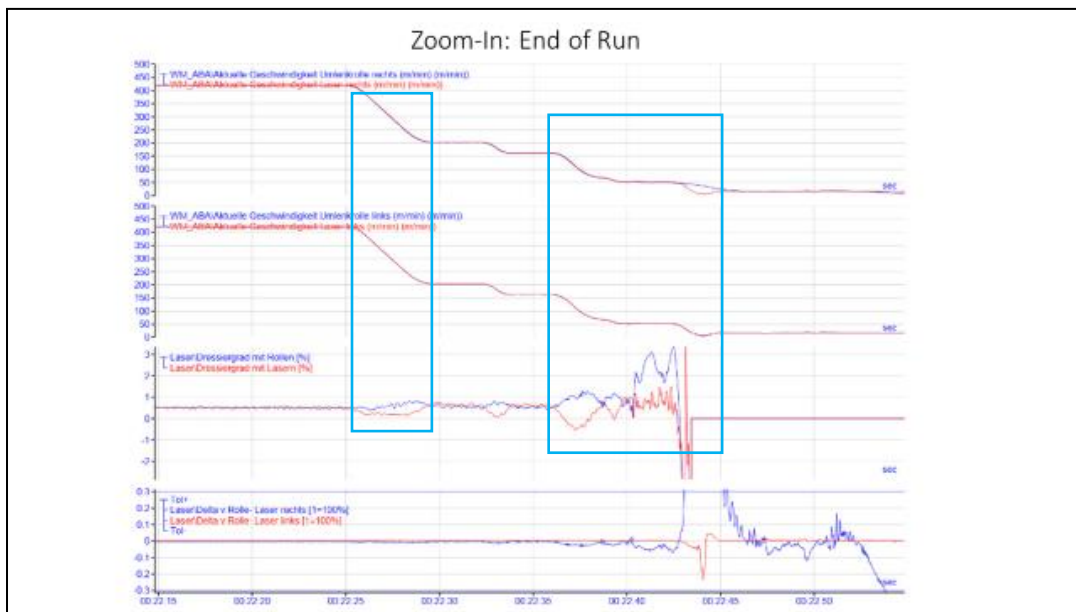
Fig. 10b: Graph describing the end of a run
