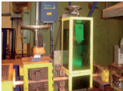
Two of the installed LSV-300 Surface Velocimeters for cut-to-length control at Mueller Copper Tube in Bilston, Great Britain.
