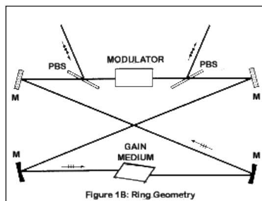
The temporal pump profile of the gain medium is considered to be CW if appreciable gain exists in the cavity for an appreciable time before the pulse to be amplified is injected and begins to increase immediately after the amplified pulse is extracted. Conoptics offers drivers for both CW pumped and non-CW pumped amplifiers.
