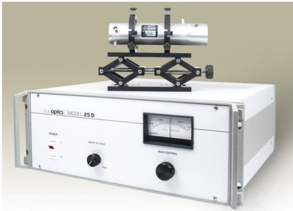
Conoptics series of electro-optic beam deflectors utilize a quadrupole electric field in an electro-optic material to produce a linear refractive index gradient proportional to the applied signal voltage. Choice of the proper material and crystallographic orientation eliminates piezoelectric ringing normally associated with other deflectors. There are no moving parts and they do not fatigue with prolonged use.
