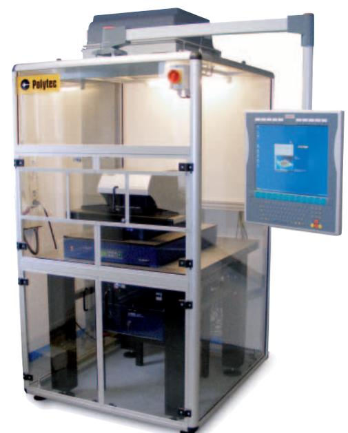
Fig. 5: Workstation for TopMap White-Light Interferometer.
