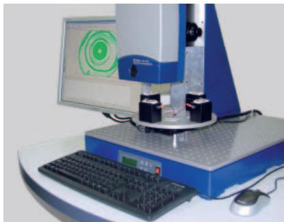
Fig. 2: TopMap In.Line White-Light Interferometer.
