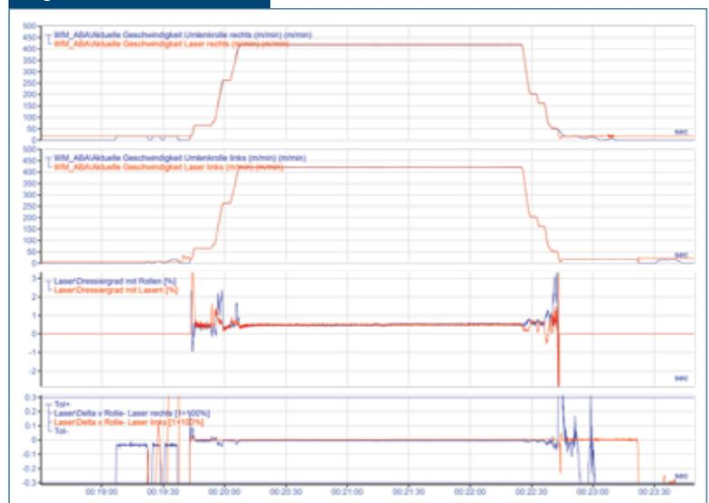
Mill entry/exit speed and elongation: (LSV in red: deflector roll in blue).
