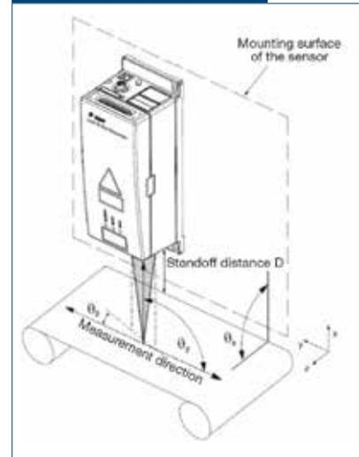
Positioning of the sensor head.
