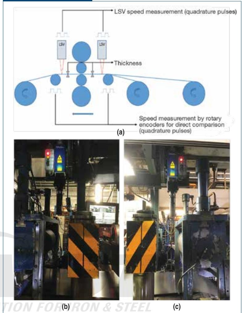
Schematic of 4-high rolling mill (a), Polytec LSV at right side of 4-high Rolling Mill 1 (b), and Polytec LSV at left side of 4-high Rolling Mill 1 (c).
