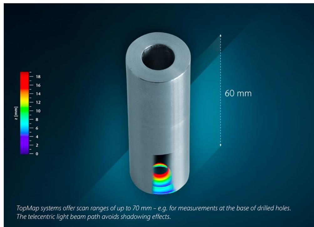
*TopMap systems offer scan ranges of up to 70 mm – e.g. for measurements at the base of drilled holes. The telecentric light beam path avoids shadowing effects.*
