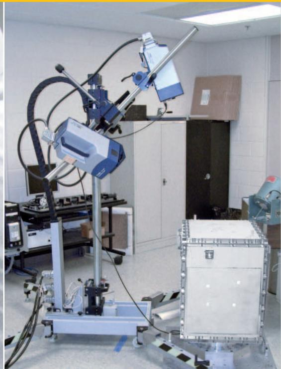
Fig. 4: FS-5 SEM II with Polytec PSV-400-3D.
