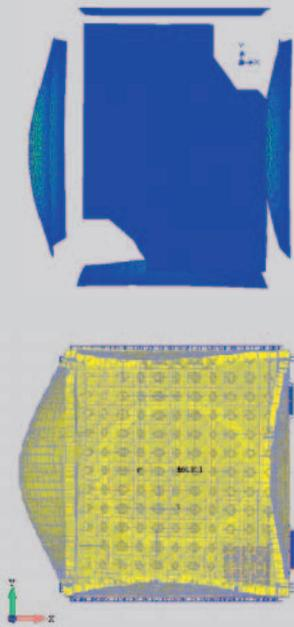
**Fig. 5: Measured mode 5 (top) vs tuned FEM – asymmetrical X panel breathing.**
