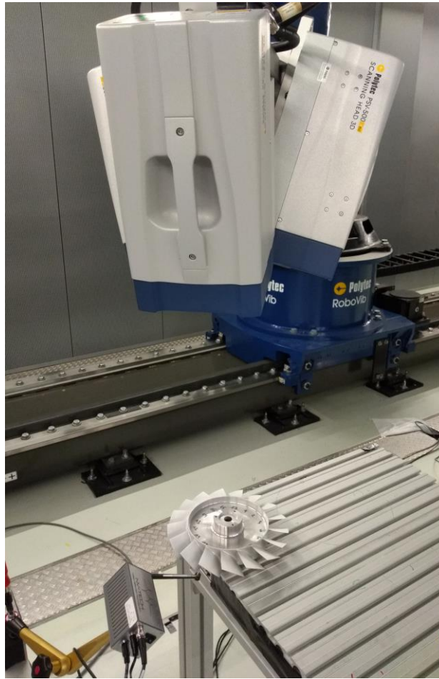
Figure 3: Experimental setup of a 17-blade turbine wheel with PSV-500-3D SLDV.
