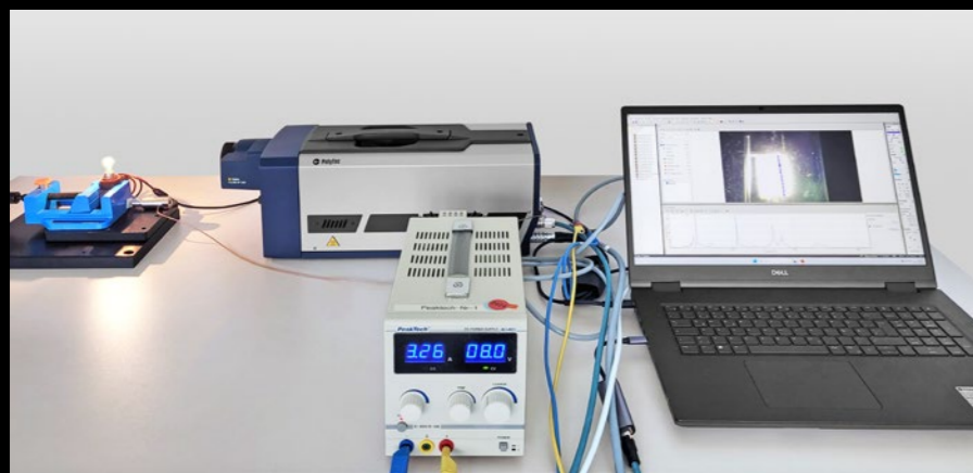
2 VibroScan Xtra QTec with Close-up Unit aligned to a light bulb
