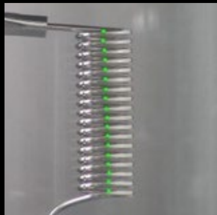
1 Filament of the measured halogen bulb. One measurement point per winding
