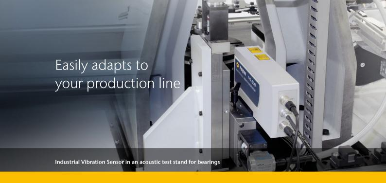
The IVS-500 comes as compact all-in-one system with decoding electronics integrated into the sensor. Several models can be selected depending on your application – from low to ultrasonic frequencies and from low to high velocities. The optional auto and remote focus allow you to adapt to different sample geometries and guarantee the best signal-to-noise ratio for each sample tested.
