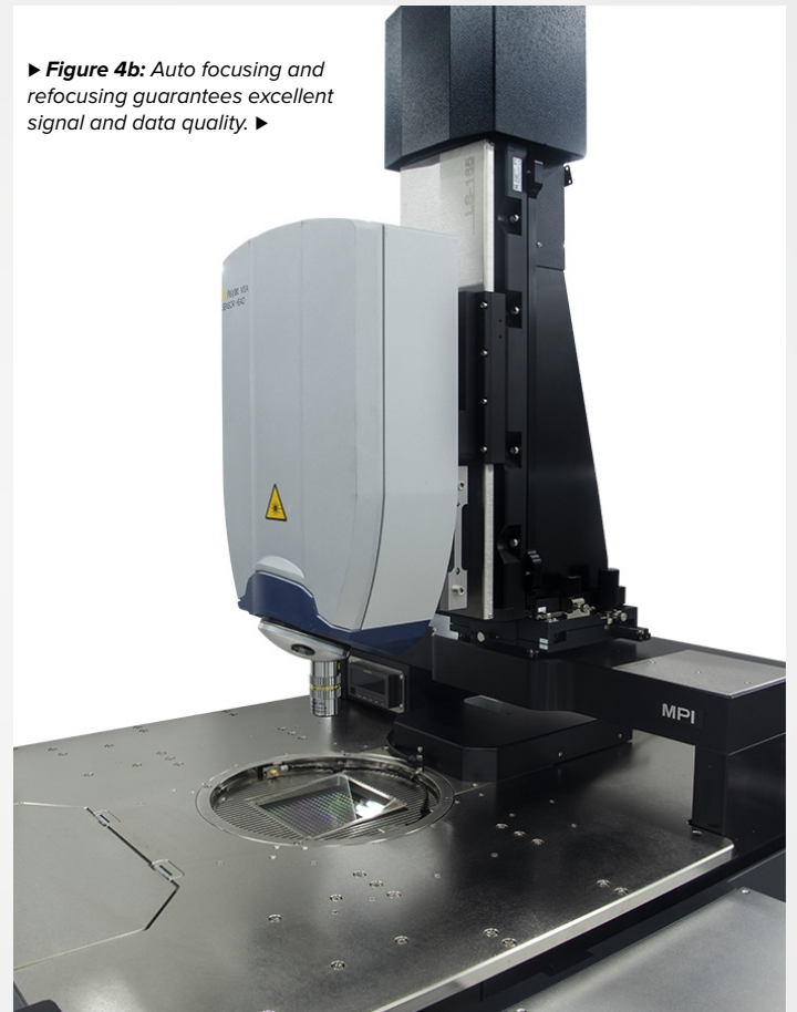
► Figure 4a: An automated test solution with HF probes for sample excitation and optical measurement head. ►
