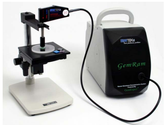
The GemExpert Raman probe with sample stage, PC with the identification programme is not shown.
